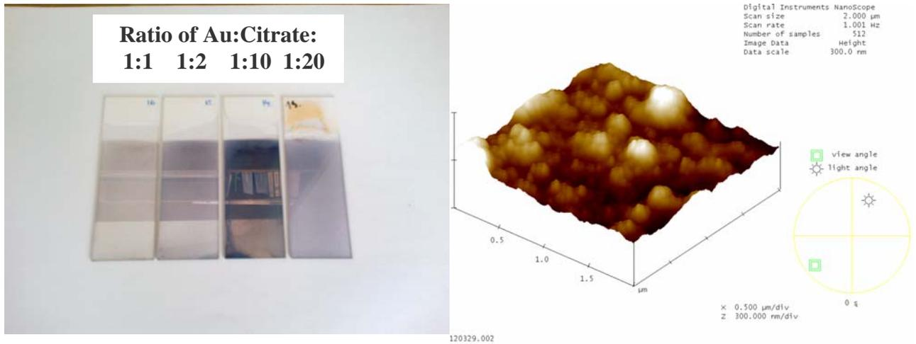
6. Fig. Photos about citrate reduced gold nanofilms on SiO<sub>2</sub> surfaces and AFM image of 5 layers film .
