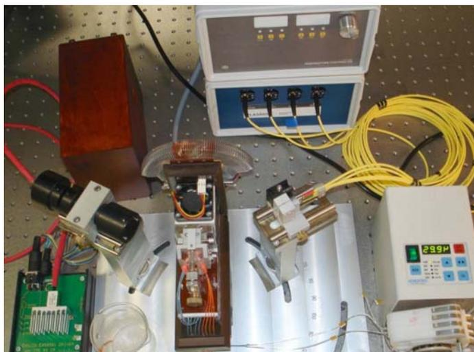
8. Fig. Plasmon II. SPR set (the resolution of set is  $2.5 \times 10^{-8}$  refractive coefficient unit).
