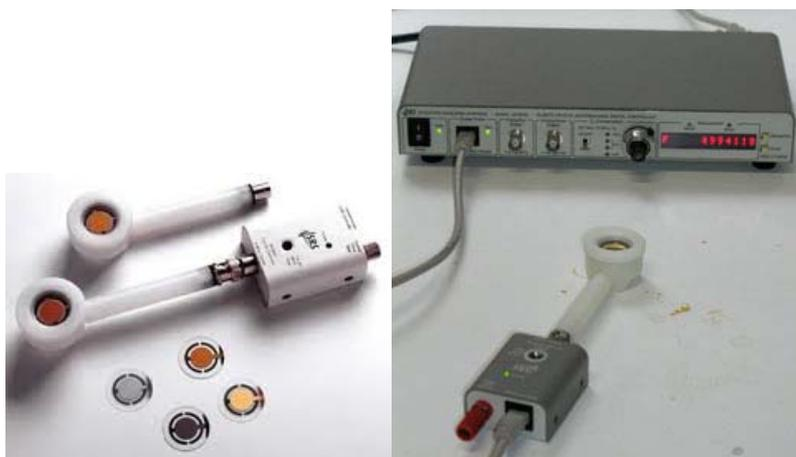
10. Fig. SRS QCM200 set and SRS QCM200 crystals (gold, silver, copper or rather platinum coating).
