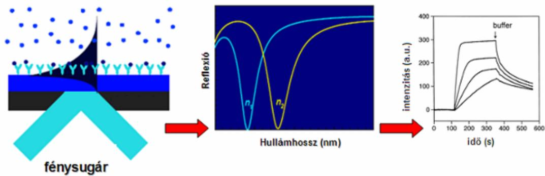
7. Fig. Schematic representation of functional disc of Surface plasmon resonance.
